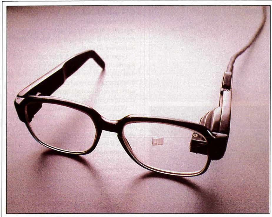
Fig. 2: Many users of the integrated version of the EGD prefer that the combiner cube be positioned high in the field of view so that the view down and horizontally forward is completely clear.
