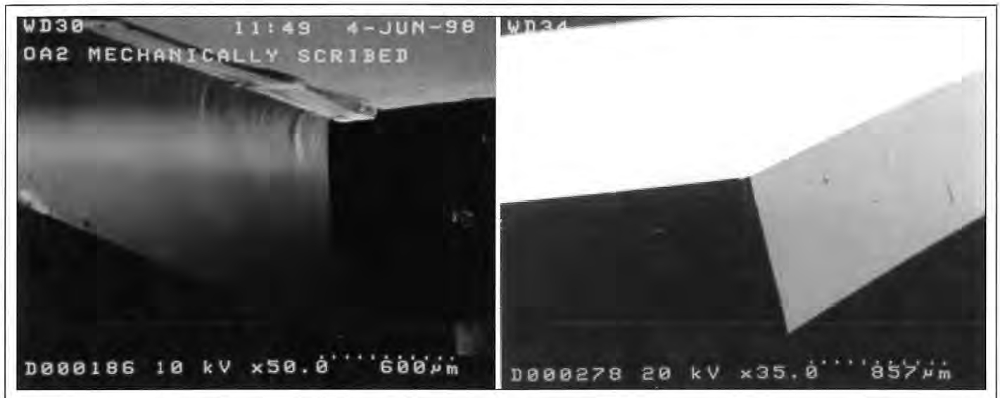
Fig. 1: A typical laser-cut edge is cleaner and more strain-free than a mechanically cut edge.
