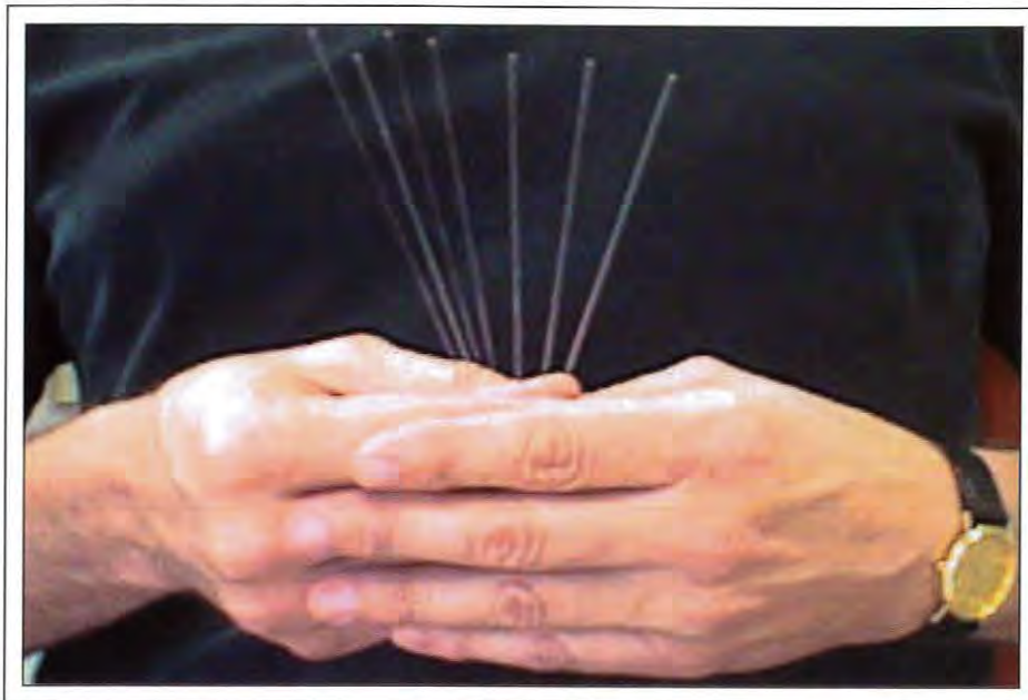
Fig. 4: With laser cutting, it is possible to cut 1.0-mm-wide strips from 0.7-mm-thick Corning 1737 glass.
