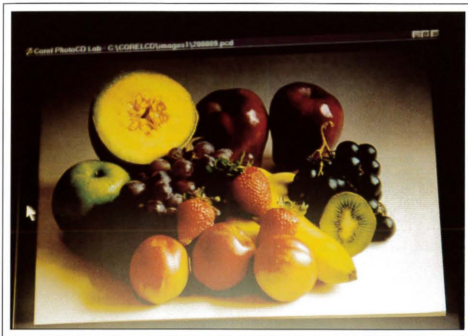
Fig. 4: This 8.4-in. SXGA SASID requires only 202 connections, compared with 3000 connections for comparable hybrid-scanned AMLCDs.
