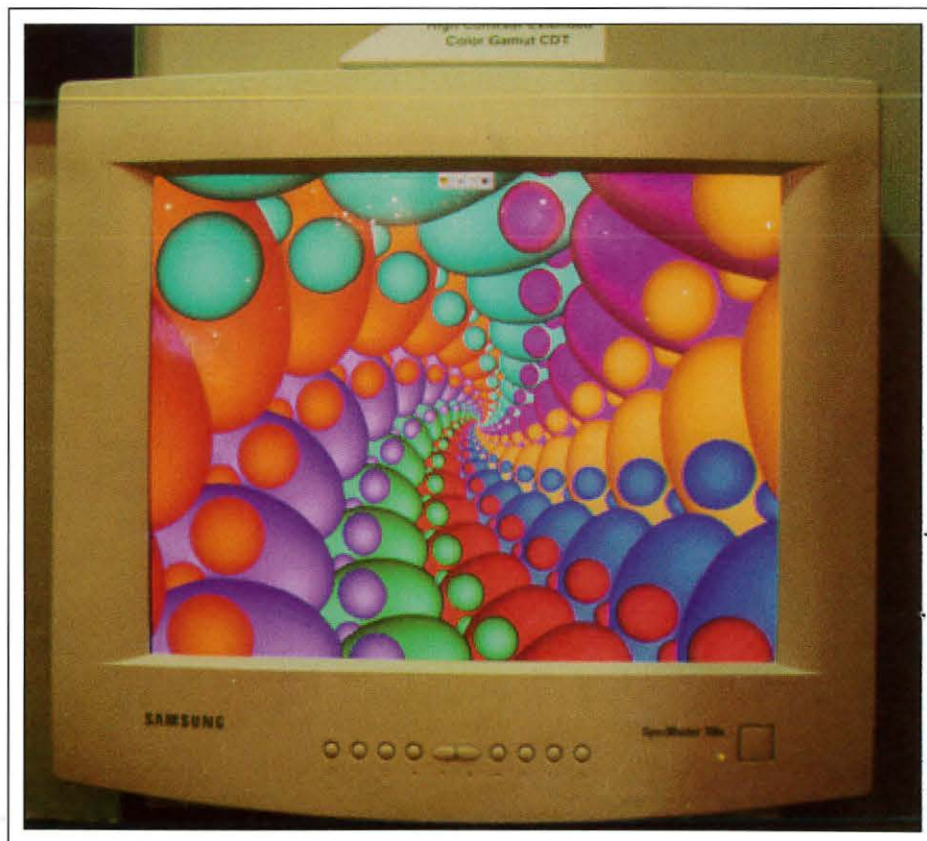
Fig. 1: Samsung's new CRT has high contrast and an extended color gamut.
