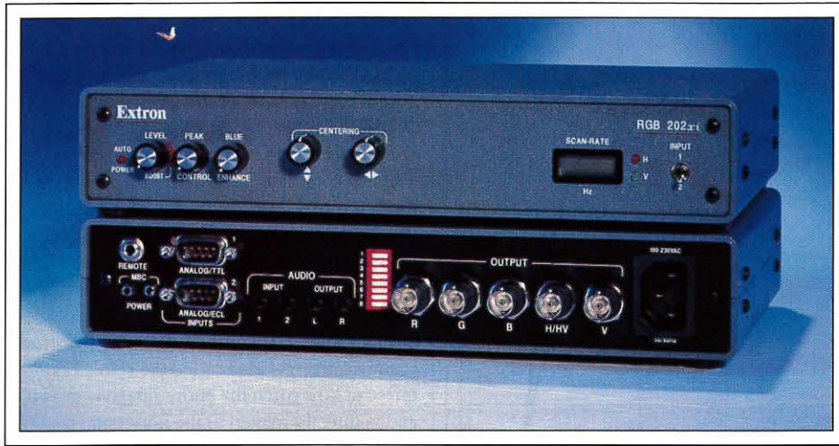
Fig. 7: A universal interface – such as Extron’s RGB 202xi – is designed to be used with many types of computer signals and cabling. Some universal interfaces, including the RGB 202xi, are also good for solving sync problems.
