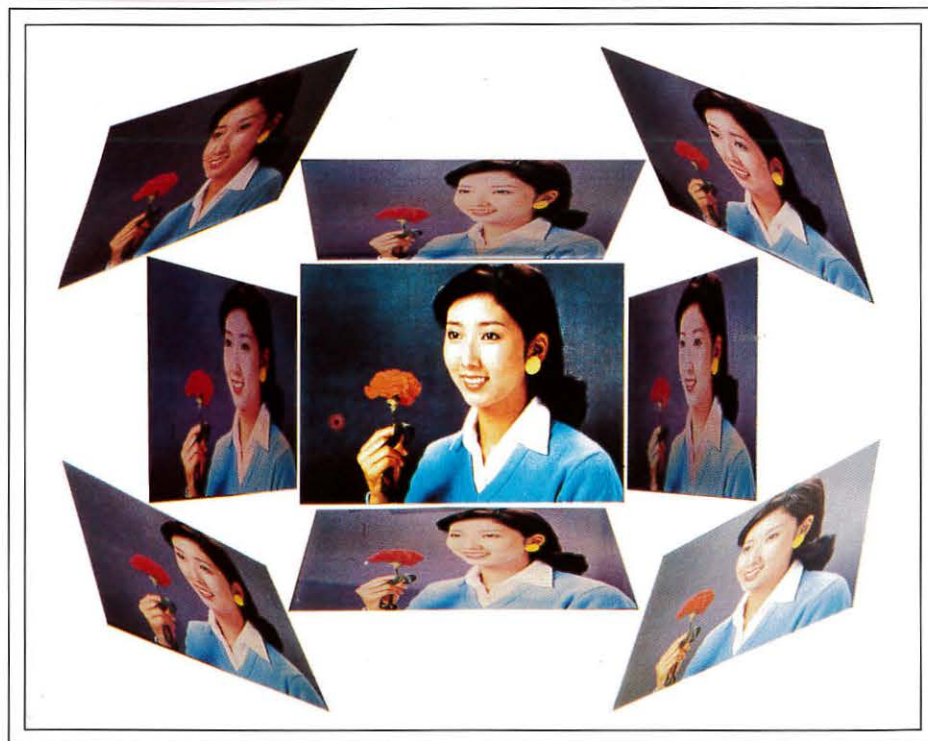
Fig. 1: Sharp's Advanced Super-V (ASV) panels have wide viewing angles in all directions.
