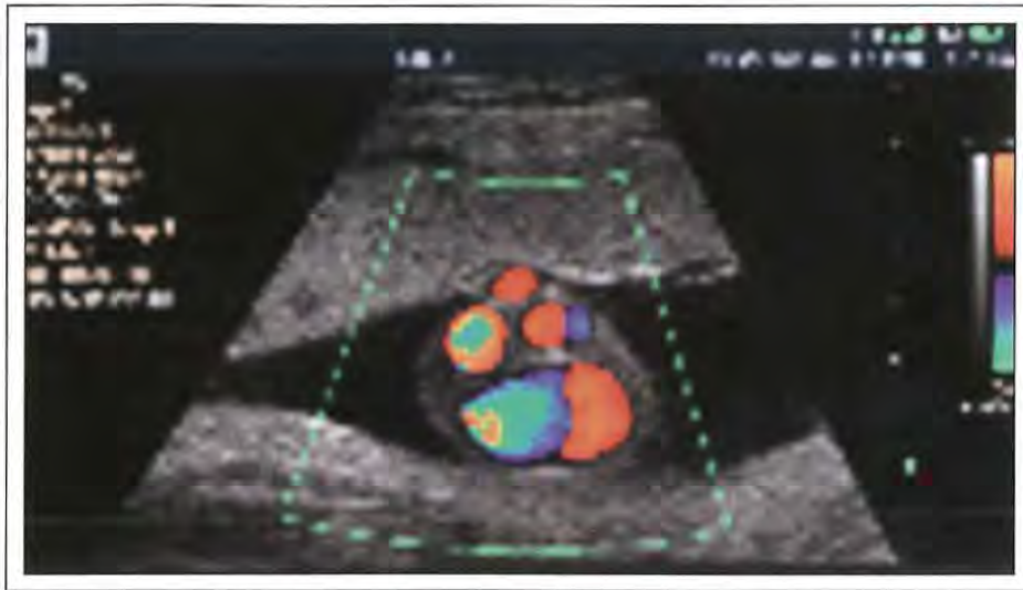
Fig. 2: The gray-image data in a typical ultrasound display is generated by a 24-bit video driver that supports 256 levels of gray. The pseudo-color data is presented with two color progressions of 128 colors that represent the direction and velocity of blood flow.
