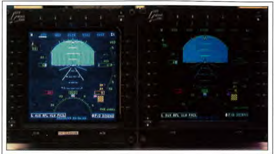
Fig. 3: A side-by-side comparison of CRT (left) and LCD (right) technologies can result in display products with better usability.
