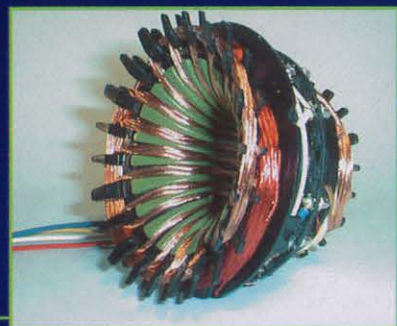
Computer-wound, patented design for high resolution medical monitors
