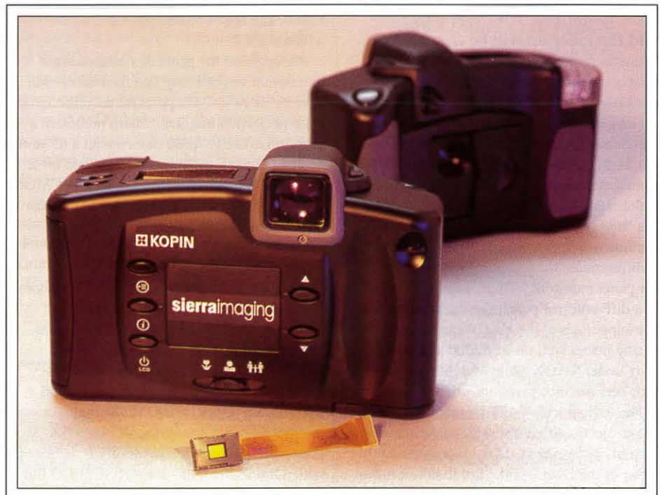
Kopin's microdisplay with transparent single-crystal-silicon TFTs is used as the viewfinder in this digital camera, and was shown in many possible applications.
