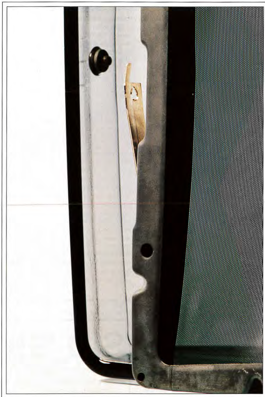
Fig. 2: This bimetallic temperature-compensating clip has been fastened to the mask frame and will be attached to the mounting lug on the CRT prior to final assembly and sealing of the CRT bulb.
