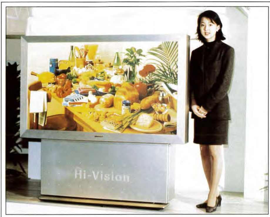
Fig. 4: This prototype of a 60-in. HDTV rear-projection receiver uses three 2.6-in. HDTV continuous-grain-silicon TFT-LCD panels.
