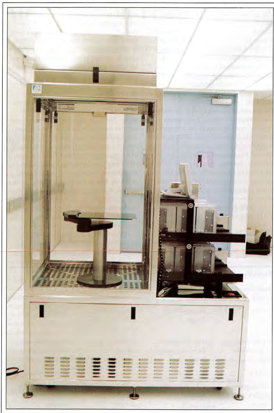
Fig. 2: A bar-type pulsed-dc air ionizer in this substrate handler greatly reduces electrostatic charges in the cassette.
