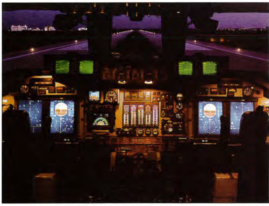
Fig. 1: The U.S. Air Force's C-141 aircraft uses rugged flat-panel-display technology for its color AMLCDs.
