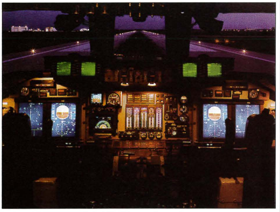
Fig. 1: The U.S. Air Force's C-141 aircraft uses rugged flat-panel-display technology for its color AMLCDs.
