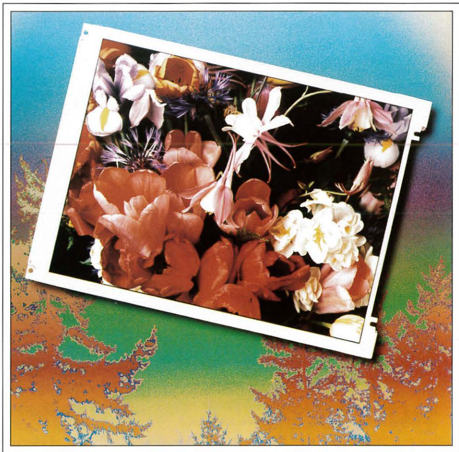
Fig. 1: At EID, Hitachi introduced its new SX3 range of high-performance-addressing (HPA) color STN-LCDs, which are fast (150 ms response time, with 80 ms coming) and have high contrast ratio (50:1) compared to conventional color STN-LCDs - at 60% of the cost of an active-matrix LCD.
