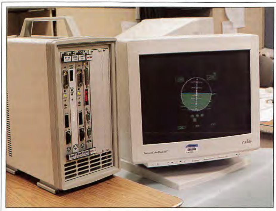
Fig. 2: A typical avionics display driven by embedded VME hardware.
