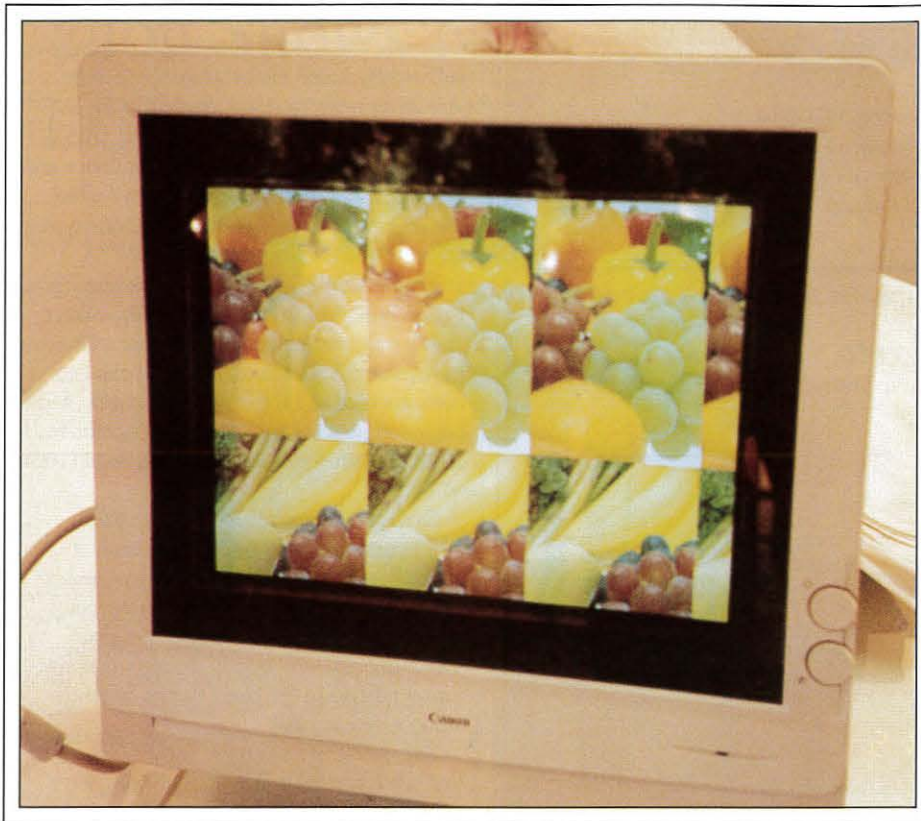
Fig. 2: Canon's prototype has new, chevron-free FLC materials. Reflections are from light bulbs in the ceiling.
