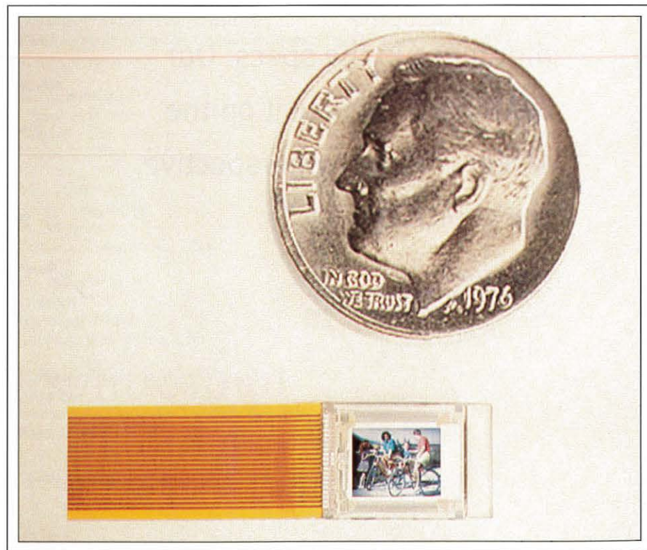
Fig. 1: The CyberDisplay 320C microdisplay from Kopin Corp. has an active display area that is only 0.24 in. on the diagonal, with 320 × 240 full-color resolution.
