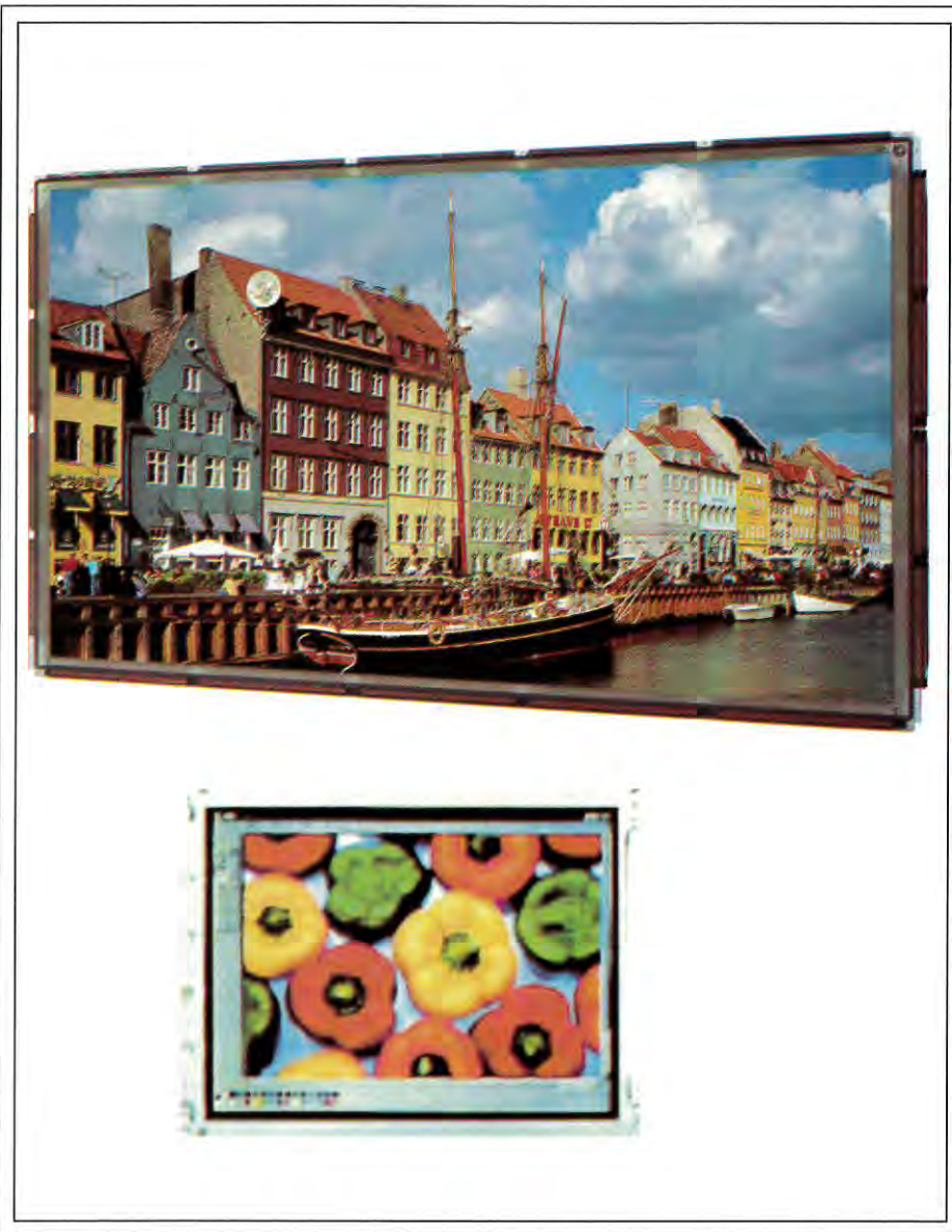
Fig. 2: The Advanced Television Systems Committee (ATSC) digital-TV specifications require a conforming receiver to support both the existing 4:3 aspect ratio (bottom) and the newer 16:9 wide-screen formats (top). The 4:3 display is Fujitsu's 15-in. XGA MVA; the 16:9 display is Fujitsu's 42-in. PDP.
