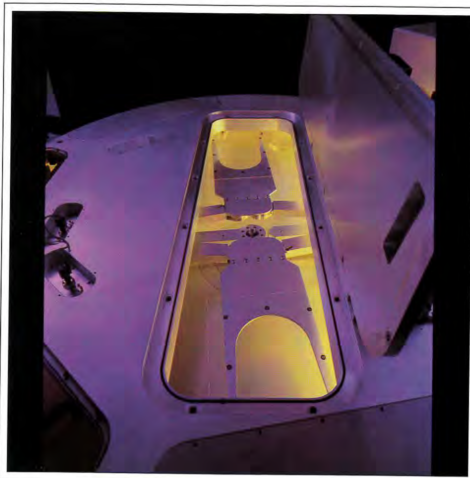
This high-throughput 600 × 720-mm transport module is for Lam Research's Continuum™ advanced FPD etch system.
