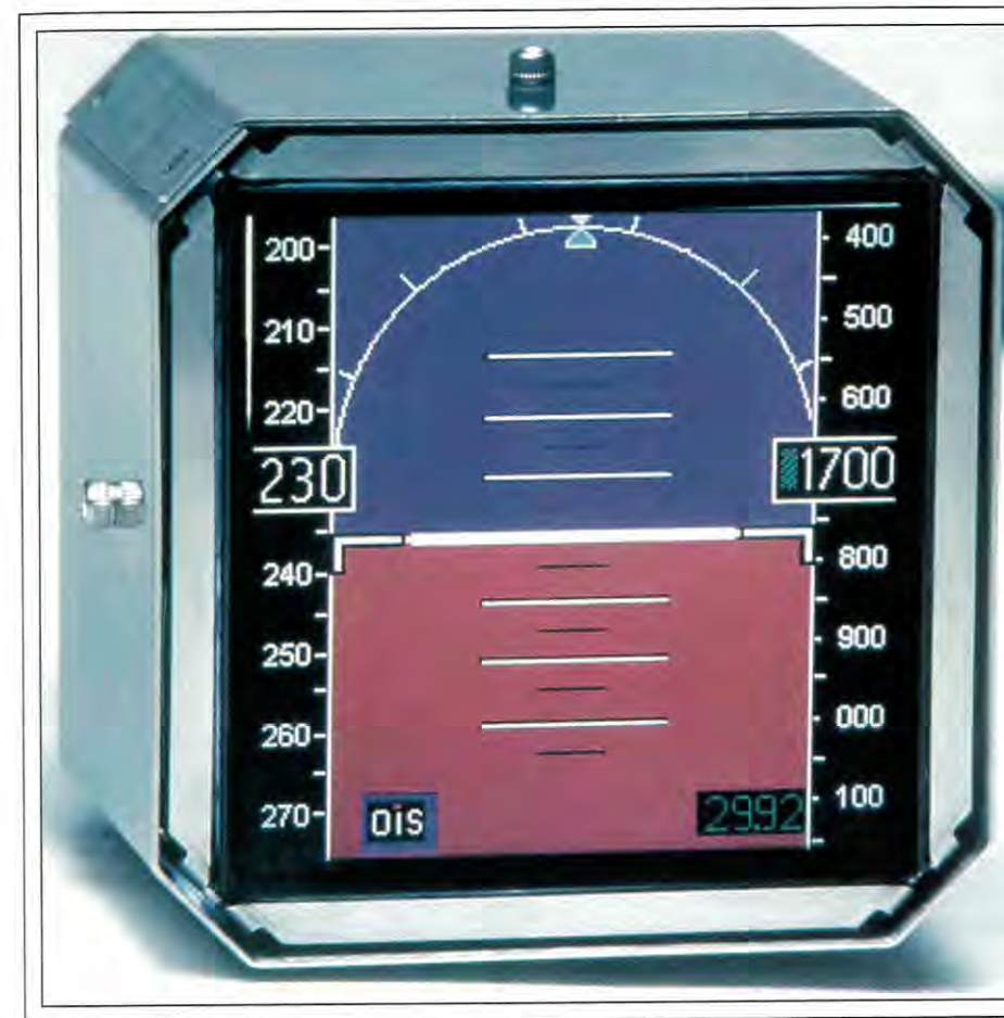
OIS exhibited this full-custom 3ATI (2.4 × 2.4 in.) AMLCD module for avionics applications.
