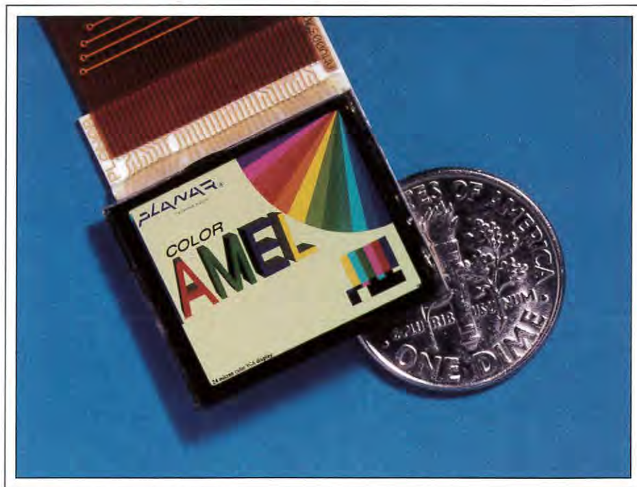
Fig. 3: Planar showed the color VGA version of its 0.75-in. 1000-lpi electroluminescent microdisplay. General sampling was scheduled for September.
