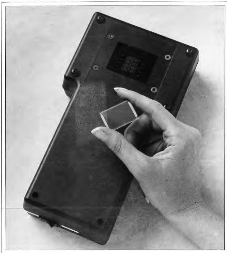
Fig. 2: Uniax Corp. premiered its organic light-emitting polymer (OLED) character and graphics displays at SID '97.
