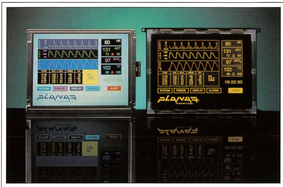
Fig. 2: Planar's IceBrite™ and ColorBrite™ electroluminescent displays looked huge next to the new 0.7-in. MicroBrite™ color AMEL (not shown in this photo).
