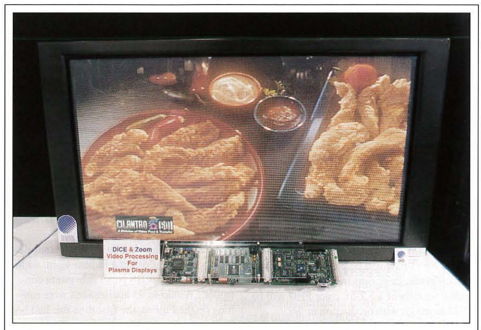
Fig. 3: A controller based on Genesis Microchip's DICE line-doubler chip and gm833x3F scaling chip zoomed a digital video source to fill the screen of this Fujitsu 42-in. PDP.
