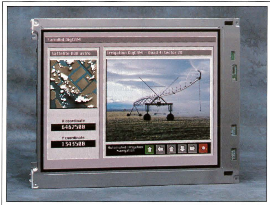
Fig. 3: Sharp's new LM12S02 multi-line-addressed 12.1-in. STN-LCD module offers 150-ms response time, 40:1 CR, and 260,000 colors – without TFTs.
