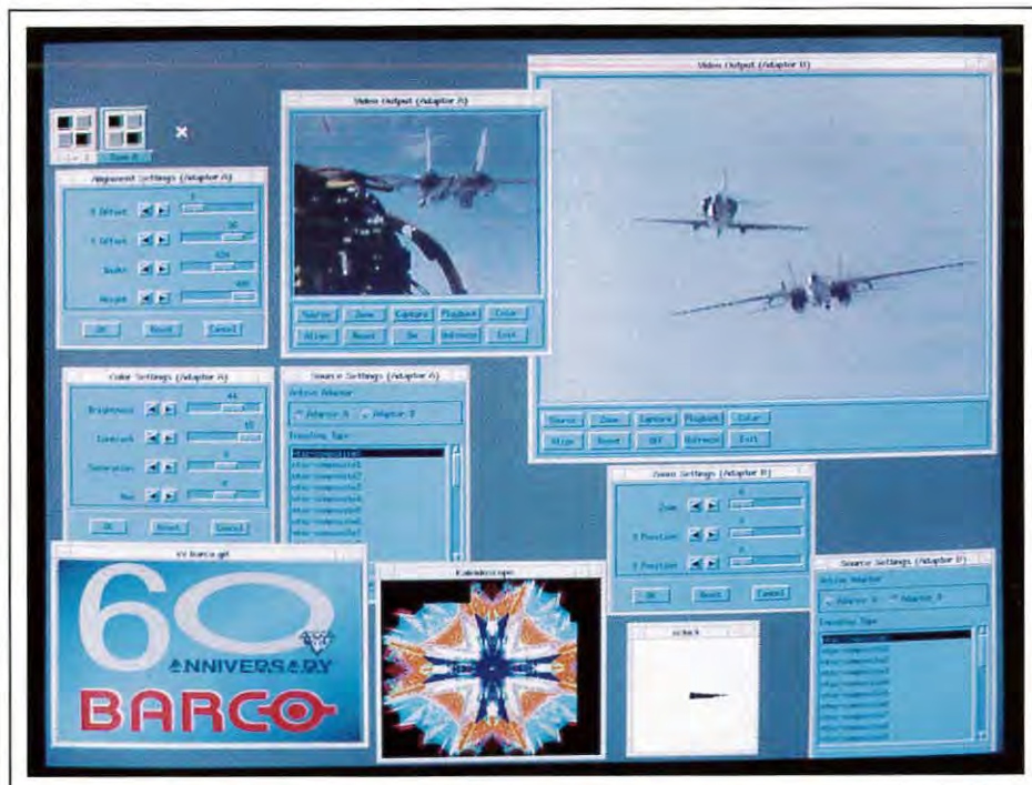
Fig. 1: If we could keep fast-scan and slow-scan systems separate, life would be relatively simple. But there is an ongoing requirement in color graphics/video systems to mix the two scanning technologies, such as when video data is used with GUIs in mission planning and control systems.
