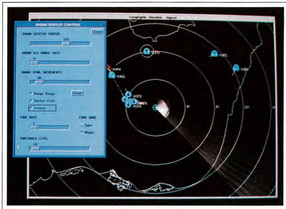
Fig. 5: In the adaptive line-doubling technique, the scan converter switches between line repetition and field repetition on a pixel-by-pixel basis. As a result, images from electronic sources are rendered with a quality that is better than the 15-kHz video displayed on a standard-resolution CRT.
