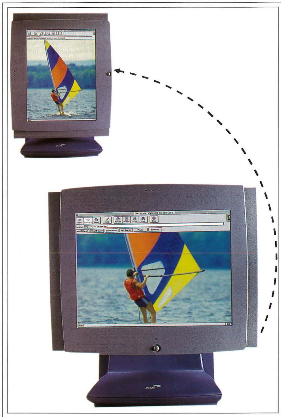
Fig. 3: Among the hundred-odd LCD monitors shown at Computex were several that rotated to convert from a landscape to a portrait display. Among them was ADI's 13.3-in. TFT-LCD monitor.
