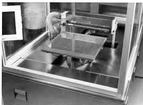
Stand Alone Non-Contact Dry Cleaning Module: Eliminates 95% of particles greater than 1 micron. High frequency pressure waves from an ultrasonic head cause particles to vibrate which are then removed by an exhaust airflow.
