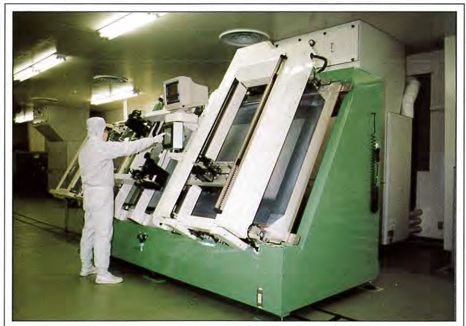
Fig. 1: Inclined PDP screen printers are more precise and occupy less floor space than traditional horizontal printers. This printer can accommodate screen mask frames up to 1800 × 1500 mm.
