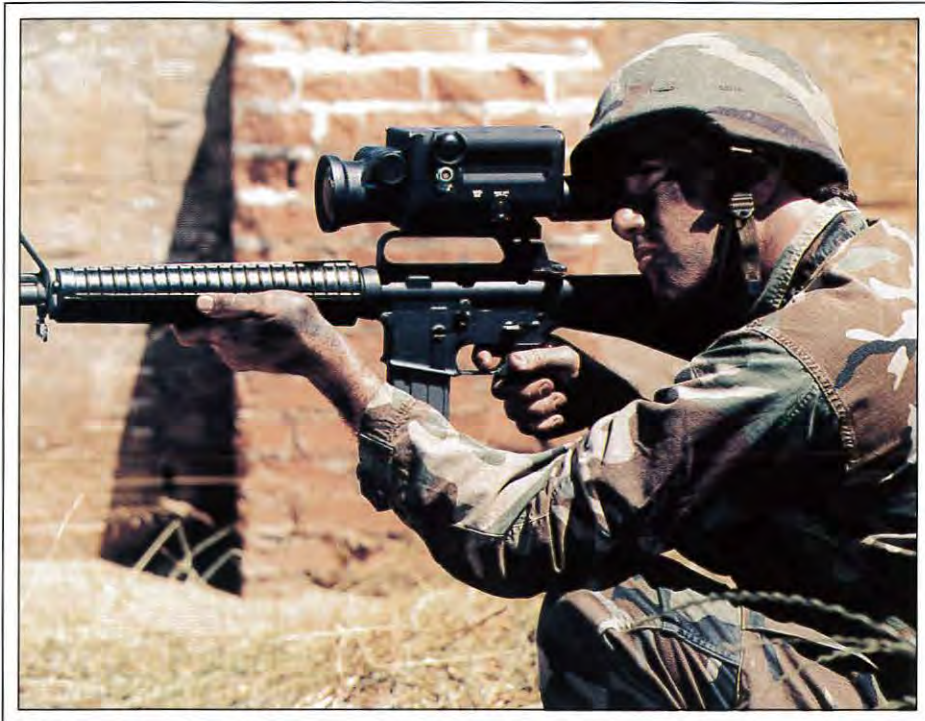
Fig. 2: Raytheon TI Systems uses neck-down CRTs in their TISIGHT, which is used on the M-16 automatic rifle shown here and the M-60 machine gun.
