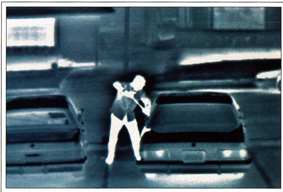
Fig. 3: The infrared image from TISIGHT's sensor is conveyed through a standard RS-170 interface to an internal monitor built around a neck-down CRT.
