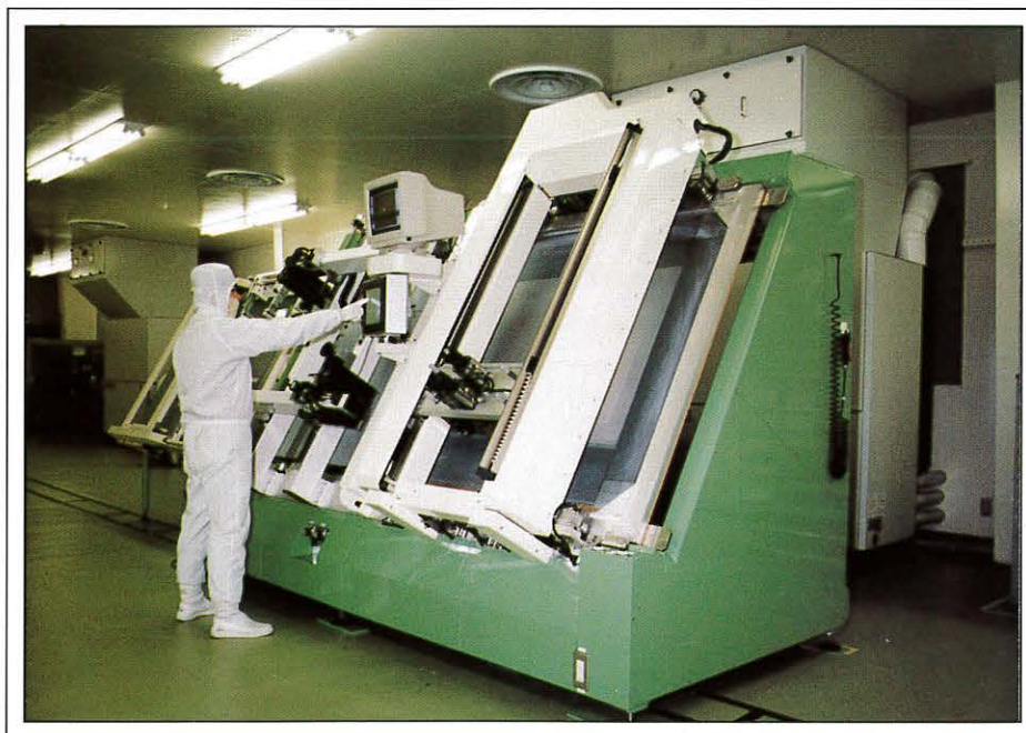
Fig. 1: Inclined PDP screen printers are more precise and occupy less floor space than traditional horizontal printers. This printer can accommodate screen mask frames up to 1800 x 1500 mm.
