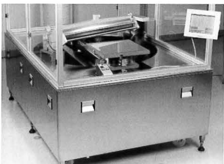
Stand Alone Rubbing Module with Rotating Table & Roller: Provides an extremely uniform rubbing action, while prolonging the life of the rub fabric. Ideal for high volume production.
