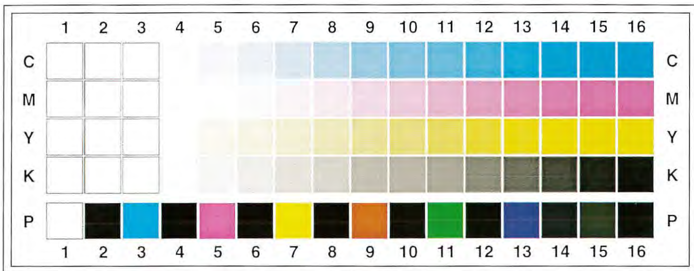
Fig. 1: Combined with its accompanying Profile/80 software, a digital target similar to this one can generate input and output device profiles for "soft proofing."
