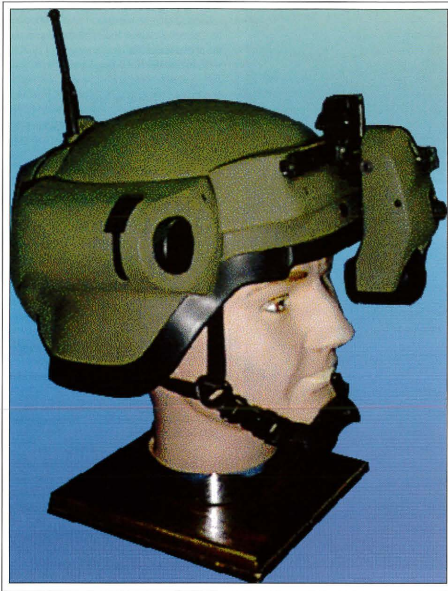
Fig. 5: The GEN II/Land Warrior Integrated Helmet Assembly Subsystem (IHAS) HMD for the dismounted soldier.
