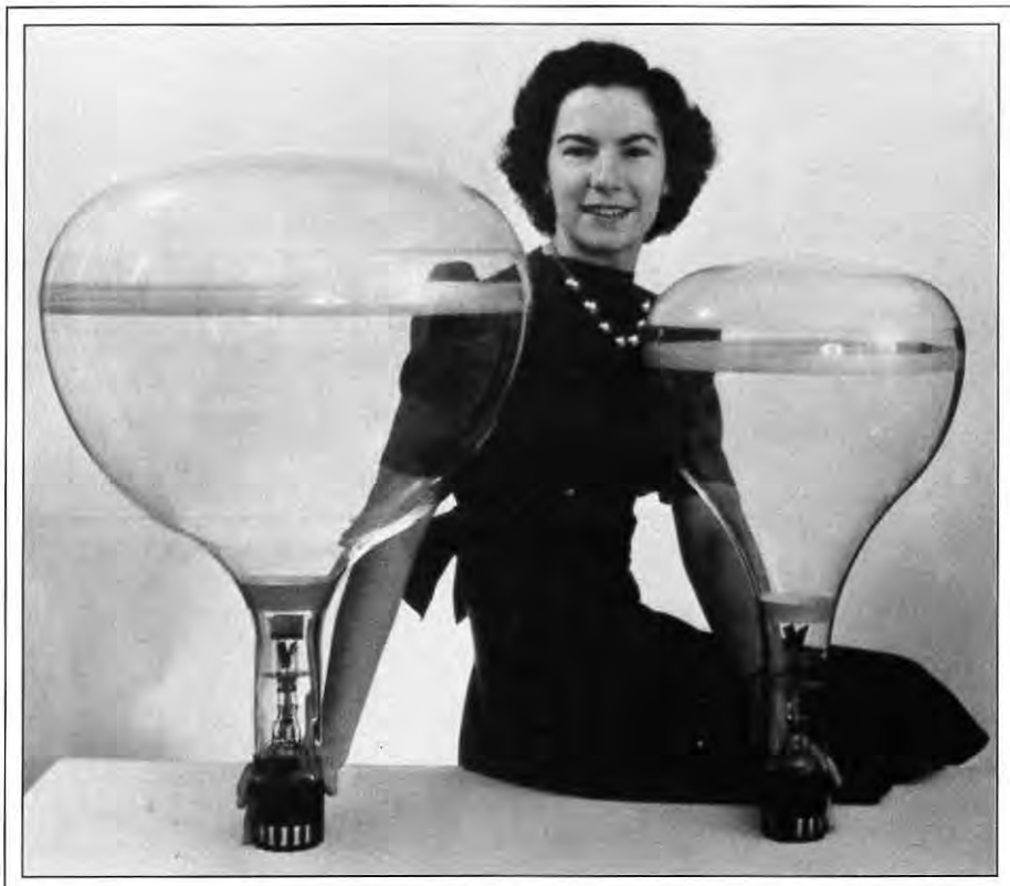
Fig. 6: Du Mont 14- and 20-in. electrostatically deflected CRTs for television. (Photograph from the Du Mont Collection at the Smithsonian Institution, Washington, D.C. Photographically copied by the author.)
