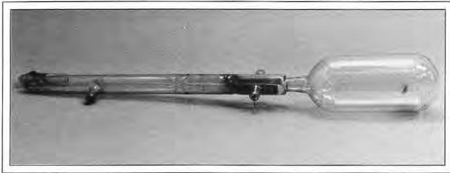
Fig. 2: Replica of the Braun CRT. (Specimen at the Smithsonian Institution, Washington, D.C. Photo by the author.)
