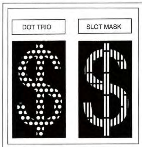
Fig. 4: Aperture-grill CRTs produce better character legibility than dot-trio CRTs.
