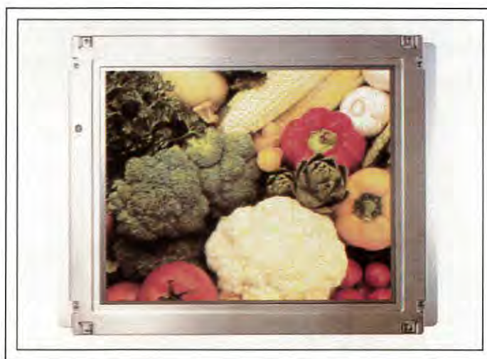
Fig. 3: IBM's 16.1-in. 1280 × 1024 (SXGA) display is now used in a variety of monitor applications. This TFT display is becoming important in non-mobile monitors.
