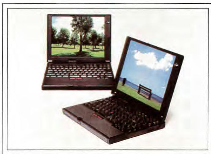
Fig. 2: IBM's strategy is that its top-of-the-line Thinkpad™ laptop computer always have a better display than its competitors. The current Thinkpad 560 family has a 12.1-in. 800 × 600 (SVGA) display.
