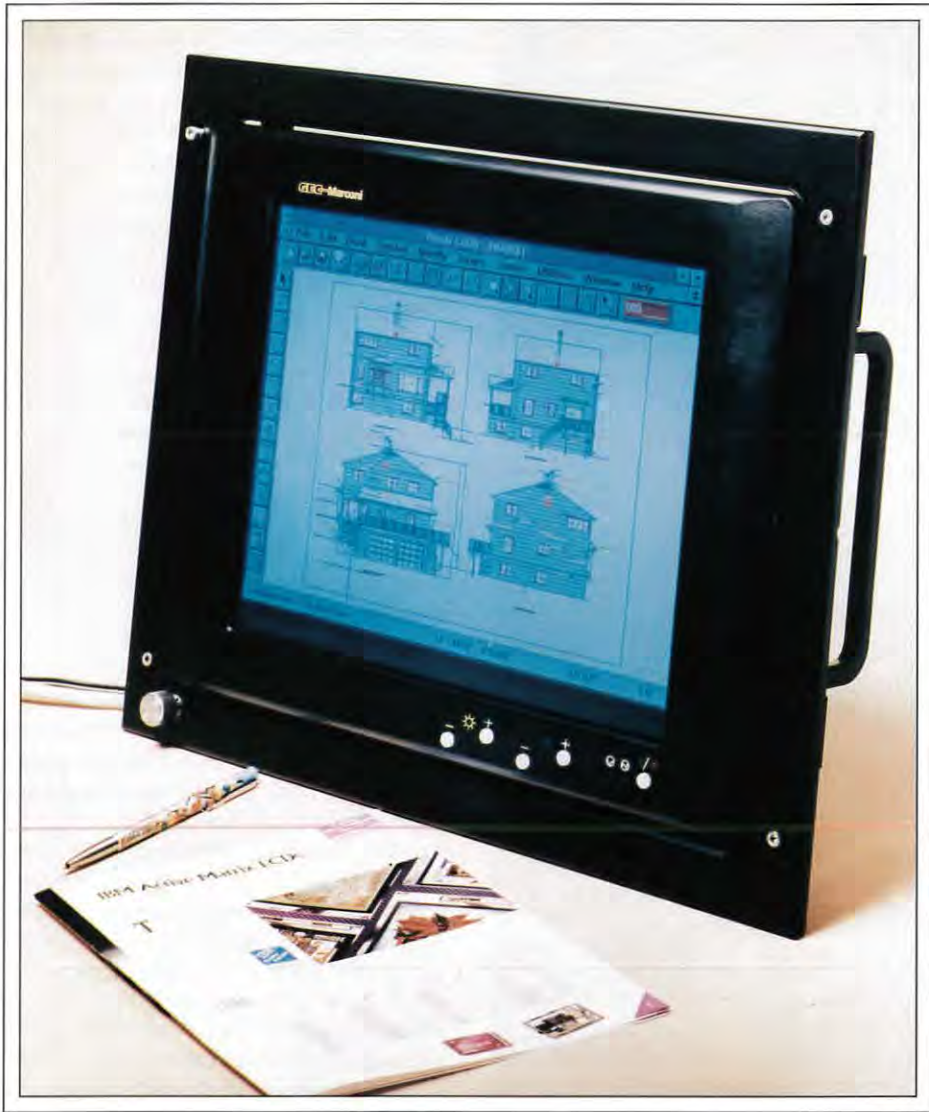
Fig. 3: The Trident-supplied IBM 16.1-in. AMLCD panel is being retrofitted by GEC-Marconi into a display console on HMS Edinburgh, a Royal Navy type-42 destroyer.
