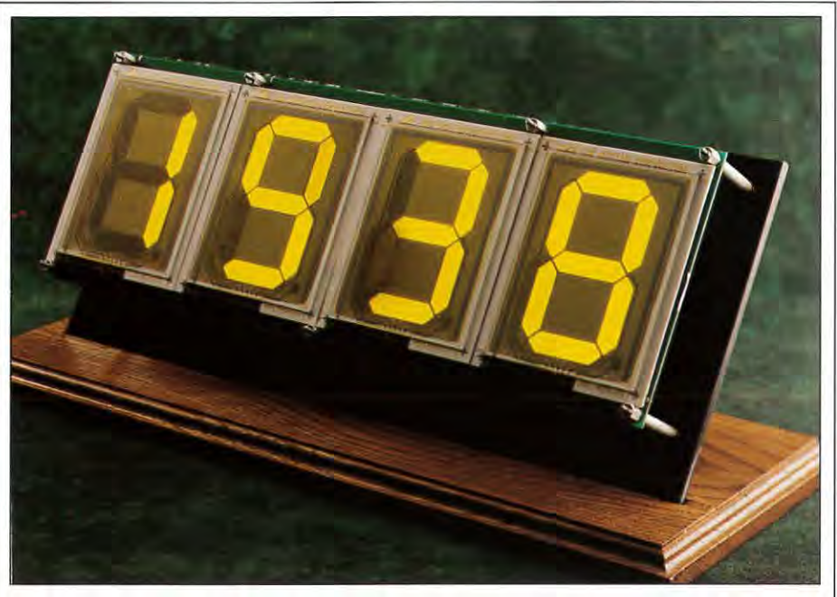
Fig. 4: TDEL technology can be used in markets where EL is not traditionally applied, such as very-large high-brightness modules for multi-segment and fixed-format displays.
