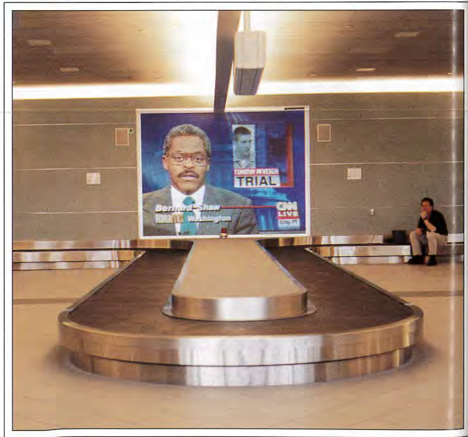
Fig. 1: A laser projector displays colors that are more saturated and subjectively brighter than conventional measurements would lead us to predict. This projector from the Corporation for Laser Optics Research (COLOR) is in the baggage area at the Manchester, New Hampshire, airport.
