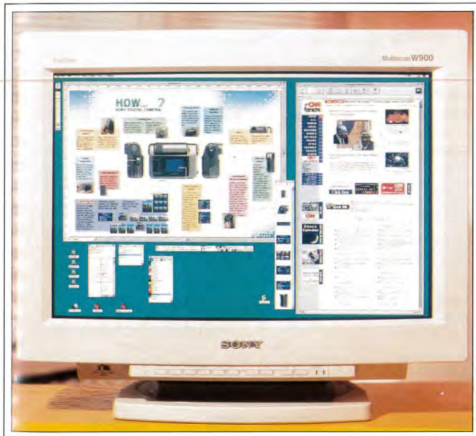
Fig. 4: Sony's Multiscan GDM-W900 monitor is built around Sony's 24-in. Trinitron tube, which has a 16:10 aspect ratio and can display up to 1920 x 1200 pixels at a 75-Hz refresh.
