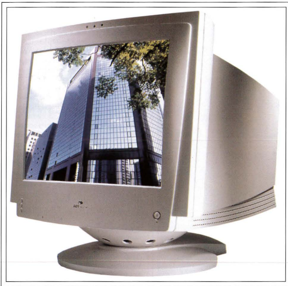
Fig. 3: ADI showed one of a surprisingly large number of prototype 19-in. color monitors using Hitachi's brand-new 19-in. flat square black-matrix Invar shadow-mask CDT.
