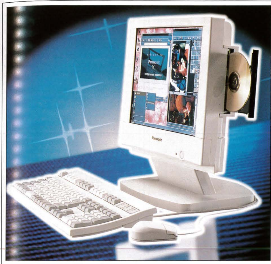
Fig. 2: Panasonic's Panel PC CF55 drew a lot of attention. The compact case houses a 14.5-in. 1024 × 768 (XGA) LCD monitor and the necessary parts of a PC, including a 150-MHz Pentium processor, two PCMCIA card slots, a floppy disk drive, and a CD-ROM drive.
