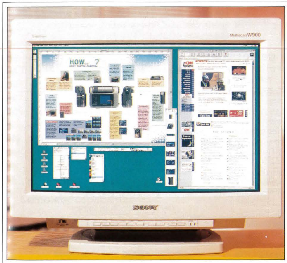
Fig. 4: Sony’s Multiscan GDM-W900 monitor is built around Sony’s 24-in. Trinitron tube, which has a 16:10 aspect ratio and can display up to 1920 × 1200 pixels at a 75-Hz refresh.
