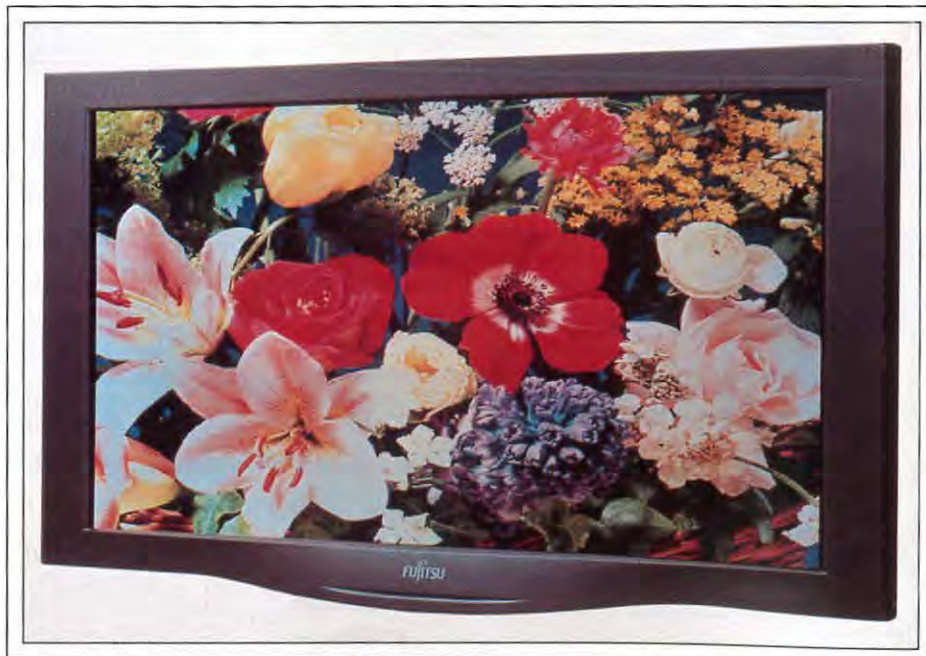
Fig. 1: Fujitsu showed the production version of its 42-in.-diagonal panel, which has a 16 × 9 format with 852 × 480 pixels and vertical color stripes.
