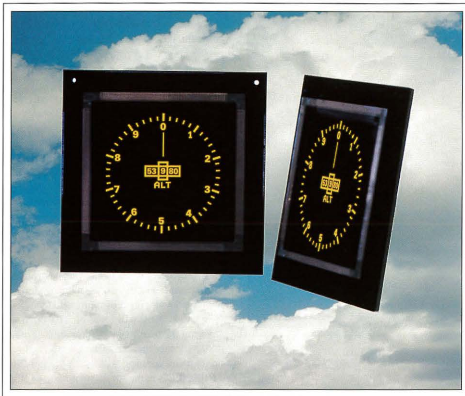
Fig. 3: Luxell was showing its sunlight-readable monochrome TFEL displays, which feature a proprietary internal "black layer" internal interference structure for suppressing reflections without external filters.
