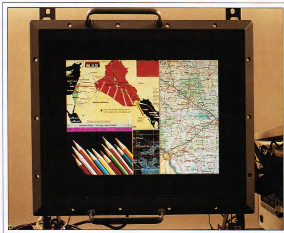
Fig. 1: The finest pixel pitch currently available in a full-color (8-bit-gray-scale) plasma display is the 0.33 mm found in Photonics' 21-in. 1280 × 1024 AC-PDP video monitor. (This display was developed with ARPA funding.)
