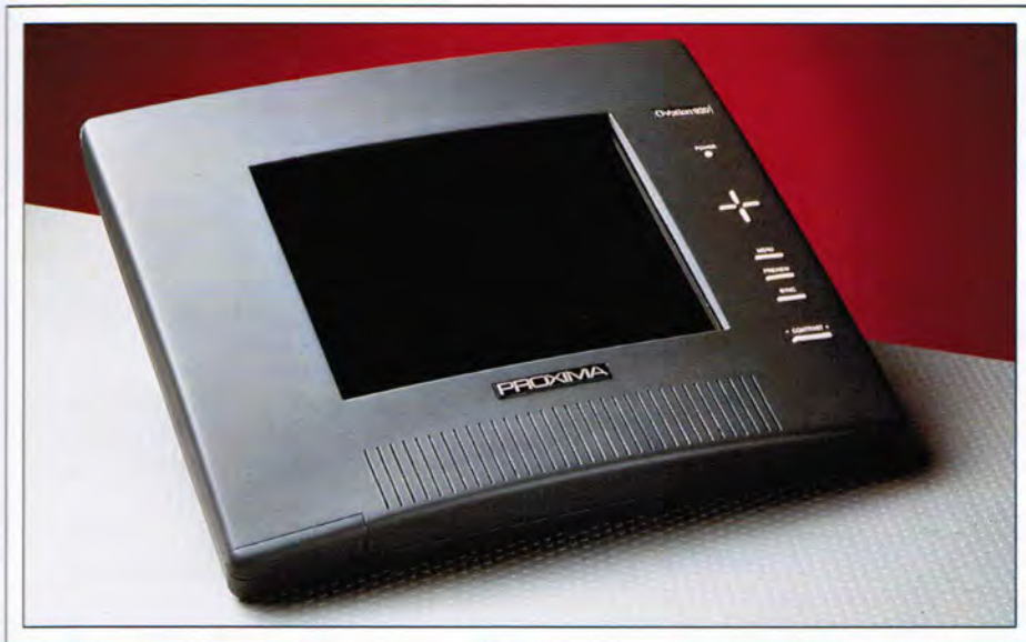
Fig. 2: The Proxima Ovation 920 panel can display 1280 \times 1024 images. Actually, there are only 1024 \times 768 pixels. It "compresses" 1280 \times 1024 images by dropping bits.
