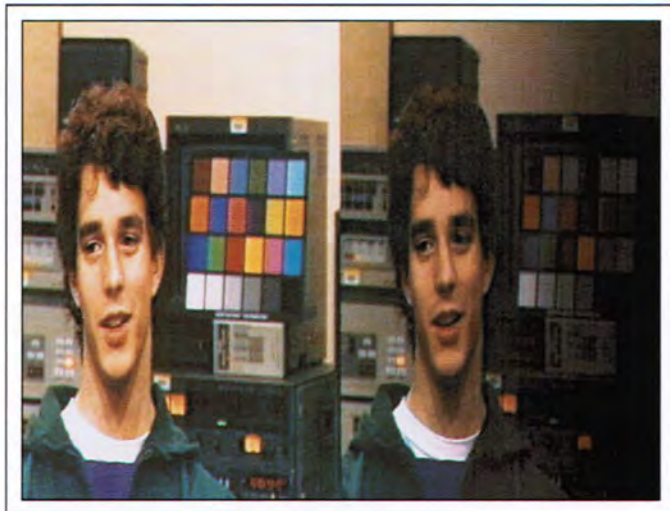
Fig. 2: The Princeton Engine has a split-screen mode that permits an original video signal to be shown on the left side of a CRT and processed video on the right side. Here, the right side shows image degradation in a transmissive LCD caused by resistance in the interconnections between TFTs horizontally across the simulated display.
