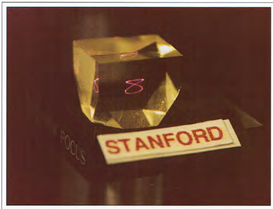
Fig. 3: A solid-state volumetric display can be based on upconversion in rare-earth-doped heavy-metal fluoride glass. When two infrared photons of different frequencies elevate an electron through two quantum states, the electron can fall back to its original state with the emission of one visible photon. The sources of the exciting photons are two lasers, and a voxel – volumetric pixel – is created wherever the two laser beams intersect. (Photo courtesy of Elizabeth Downing, Stanford University.)
