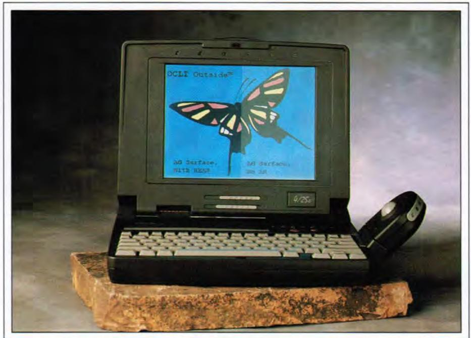
**Fig. 1:** As part of a test, an MLAR-coated polyester film was laminated to the AG surface of the polarizer on the left half of this commercially available color STN display.
