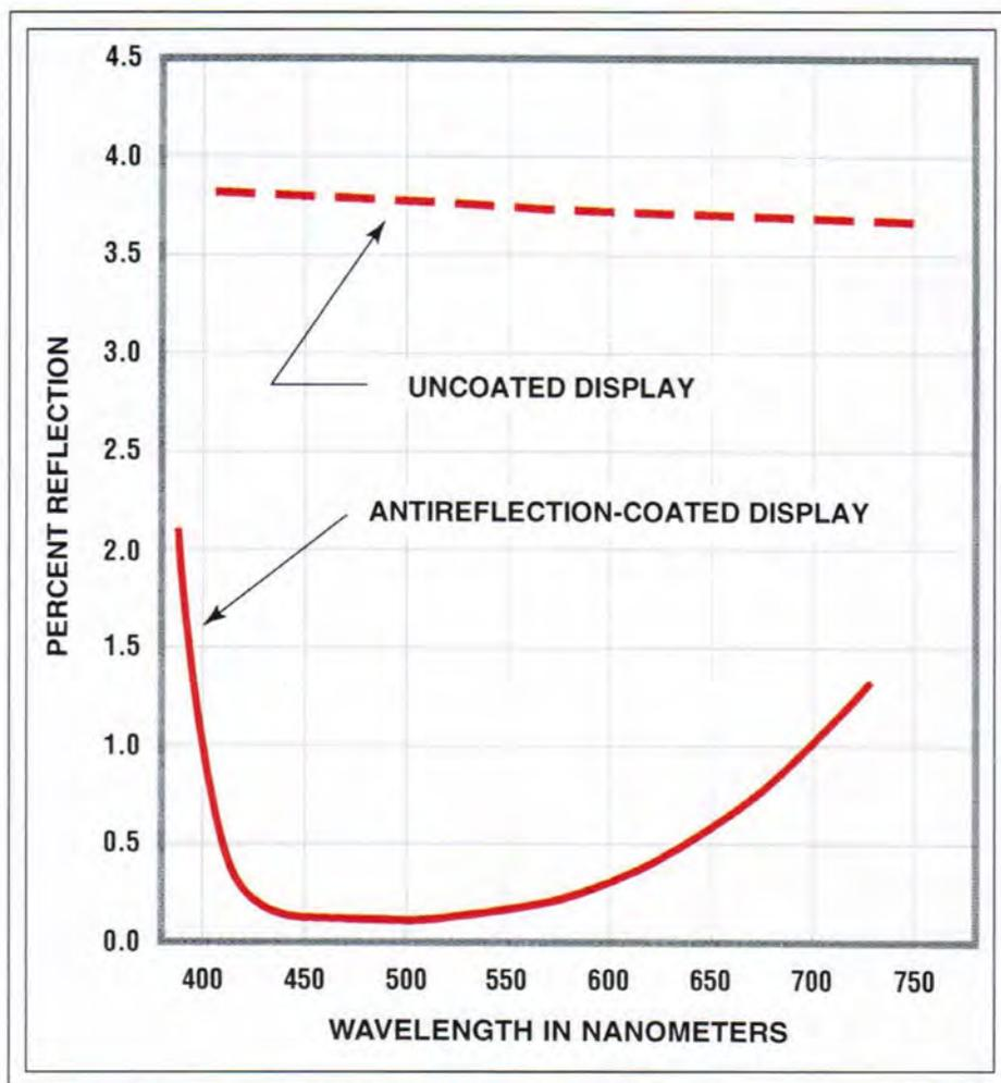
Fig. 4: Applying an MLAR coating directly to the linear polarizer prior to panel assembly reduces display reflection by nearly a factor of 20.
