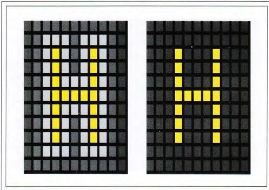
**Fig. 2:** Blooming in EL displays occurs when light emitted by a lit pixel is reflected internally and exits at an adjacent unlit pixel (left). An appropriately designed internal layer can absorb the stray light, suppress the blooming, and improve the crispness of the display (right).
