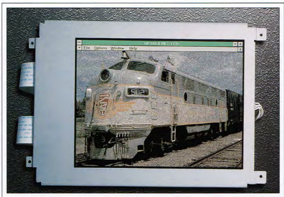
Fig. 4: Multi-Line Selection (MLS) and Active Addressing™ (AA) techniques use application-specific integrated circuits to generate addressing waveforms that allow passive-matrix displays to achieve video speeds and wide viewing angles. This MLS-addressed unit is from Optrex, the Mitsubishi-Asahi Glass joint venture. (Screen image © Second Nature Software; used with permission. Photograph by John Murray.)
