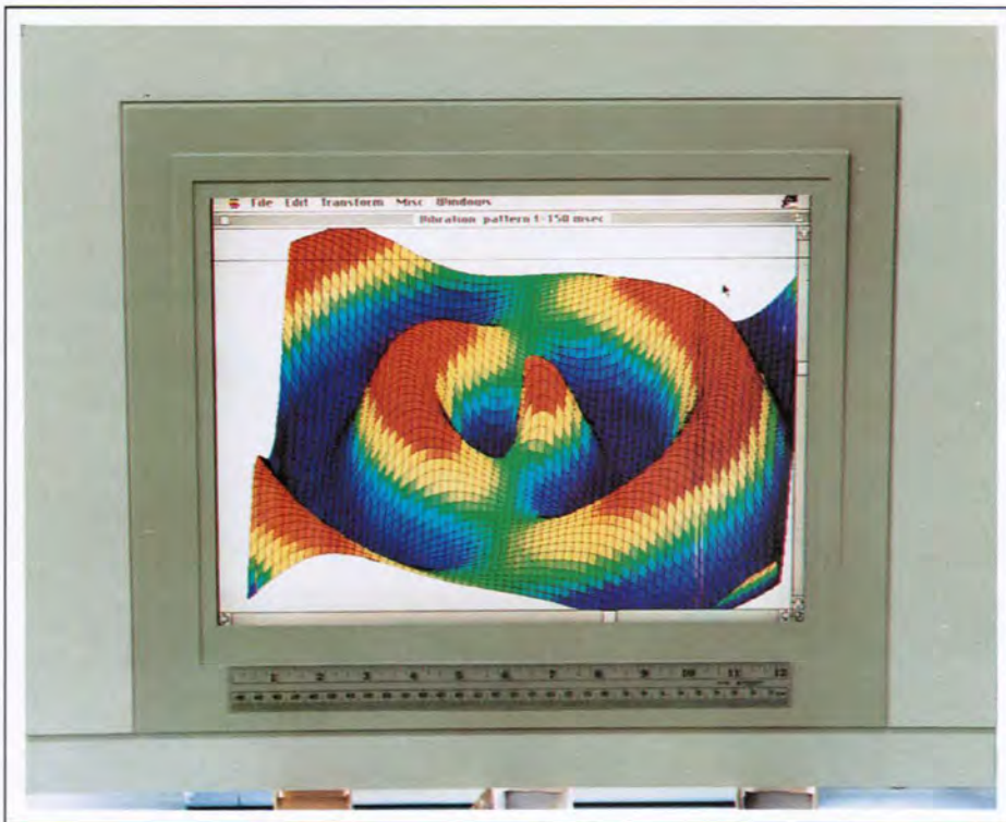
Fig. 2: At SID '93, Tektronix unveiled a bright full-color 16-in.-diagonal VGA-resolution PALCD. Plasma addressing offers the advantages of an active matrix but only requires passive-matrix tolerances, which eases the manufacturing of large-area high-resolution LCDs.
