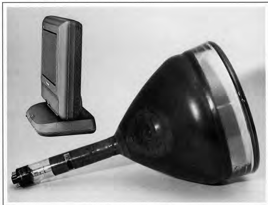
Fig. 1: The CRT's longevity has not been rivaled by any other active component because it is amenable to striking and constant improvements. A dramatic and very recent example is Matsushita's color flat-panel (CFP) display (background) that consists of a matrix-addressed array of thousands of tiny CRTs. An earlier tube that embodied important improvements was RCA Victor's 10BP4 (foreground). It solved the problem of ion burn in magnetically deflected CRTs and became the best-selling TV picture tube of the 1946-1950 period. (Photograph of RCA Victor's 10BP4 tube courtesy of Peter A. Keller, see Ref. 1.) (Photograph of color flat-panel display consisting of tiny CRTs courtesy of Matsushita Electronics Corp.)
