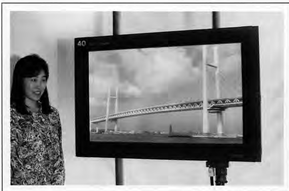
Fig. 2: Nippon Hoso Kyokai (NHK) – the Japan Broadcasting Corporation – announced a 40-in. dc-plasma HDTV display fabricated using a new high-accuracy large-area screen printer developed with Dai Nippon Printing Co.
