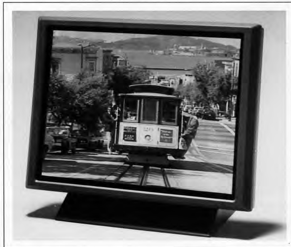
Fig. 1: The first commercial color plasma TV is Fujitsu's 21-in.-diagonal set, which uses a three-electrode surface-discharge ac-plasma display that produces an impressive peak area luminance of 200 \text{ cd/m}^2 .
