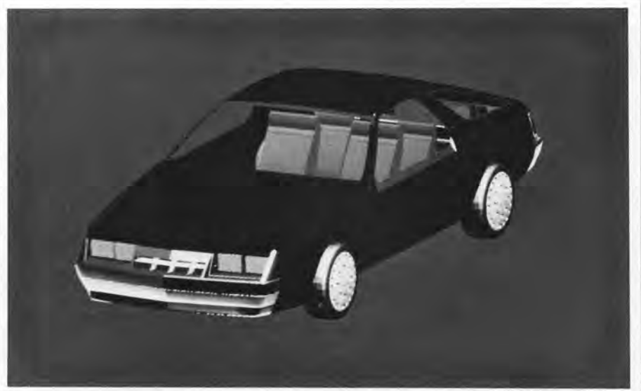
Fig. 1: The realistic rendering of complex objects such as this automobile model is easier with the extended set of "primitives" offered by the non-proprietary graphics interface system called PHIGS+. The extensions, which are not included in PHIGS itself, include shading, lighting, and advanced curve and surface commands. PHIGS is about to become an ANSI standard. PHIGS+ is under development.
