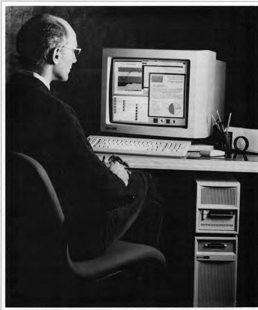
Fig. 1: Today's de facto standard workstation display is based on a 19-in.-diagonal full-color shadow-mask CRT and has sufficient resolution for an effective windowed user interface.
