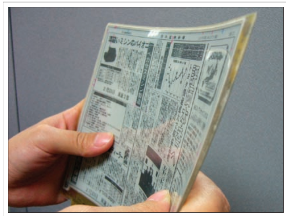
Fig. 4: This 9.7-in. EPLaR display is flexible, though not rollable.
