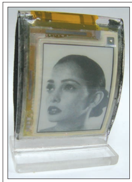
Fig. 5: This 1.9-in. EPLaR display in a curved holder can hold this shape indefinitely.
