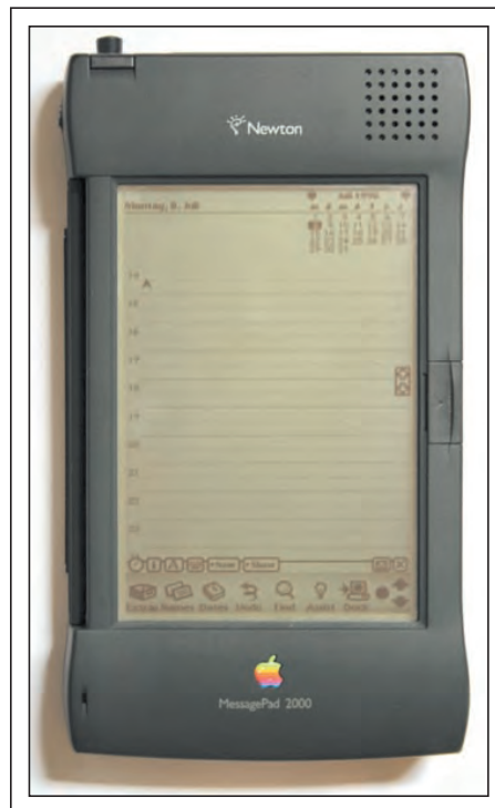
Fig. 2: The Apple Newton was the first handheld, battery-operated electronic device to utilize a large (4.5-in. diagonal) touch-enabled display when it was introduced in the early 1990s. Copyright Ralf Pfeifer, 2005.
