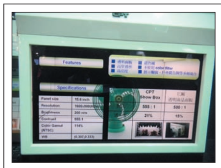
Fig. 5: CPT's shadow-box transparent display is being demonstrated for signage applications.
