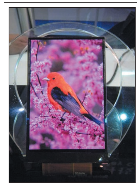
Fig. 6: RiTDisplay's 3.5-in. AMOLED HVGA panel uses an active-matrix backplane from Ignis Innovation.
