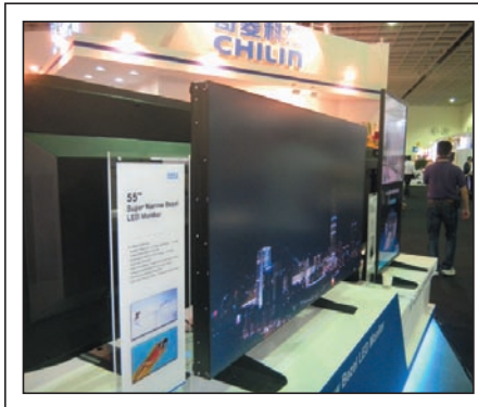
Fig. 7: ChiLin's 55-in. narrow-bezel tiled LCD has a "pencil-thin" image-to-image gap.
