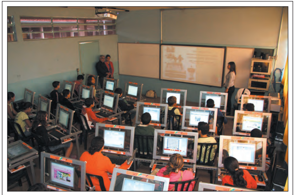
Fig. 3: This Serrana public classroom is fully equipped with Digital Desks, air-conditioning, and a digital board at the front of the room. Students in this picture are using the multi-terminal version: one computer is a server for five desks. The digital board at the front of the classroom is based on a projector (courtesy of the city of Serrana). The table tops can also be put in horizontal position during operation, to ensure a clear line of sight between teacher and student.
