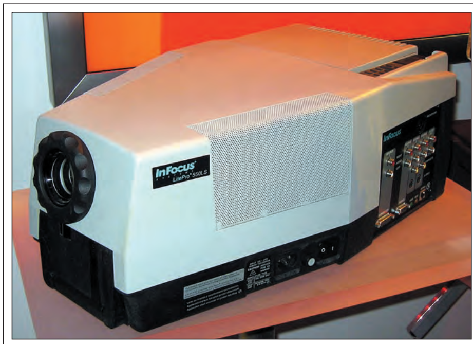
Fig. 17: The InFocus LitePro 550LS from 1998. This VGA projector used a 400-W halogen bulb, produced 130–155 lum, and was intended to replace an overhead projector.
