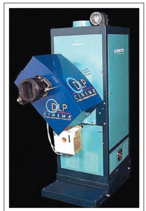
Fig. 14: DLP projector used in the 1999 digital-cinema tests mounted on a Christie xenon-lamp lighthouse originally designed for a film projector.
