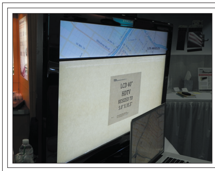
Fig. 5: Tannas Electronics can cut LCD panels to create displays with novel dimensions. Photo courtesy of Alfred Poor.
