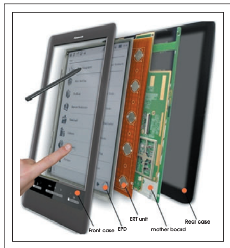
Fig. 5: In Hanvon's dual-mode (pen and finger) EMR digitizer, the sensor board (labeled "ERT unit") is shown inserted between the electronic-paper display (EPD) and the motherboard in an e-Reader. The circles shown on the sensor board represent one column of an array of force-sensing piezo capacitors. Image source: Hanvon.
