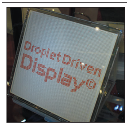
Fig. 4: ADT showed, for the first time, a highly pixelated and bistable droplet-driven (electrowetting) display.
