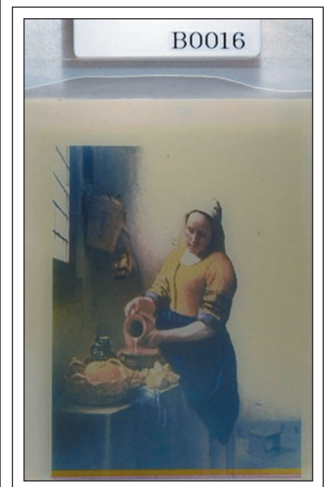
Fig. 3: Ricoh unveiled a three-layered (CMY) electrochromic display capable of 70% white-state reflectance and, amazingly, driven with a single backplane.
