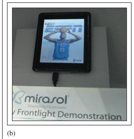
Fig. 2: (a) External ambient illumination is used (as it would be for standard e-Paper) and (b) the display in a dark environment with the front light activated.
