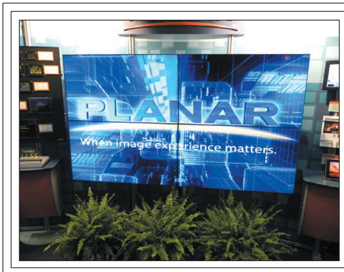
Fig. 2: Planar’s LCD panels have thin bezels so that they can be tiled to create a video wall. Photo courtesy of Alfred Poor.
