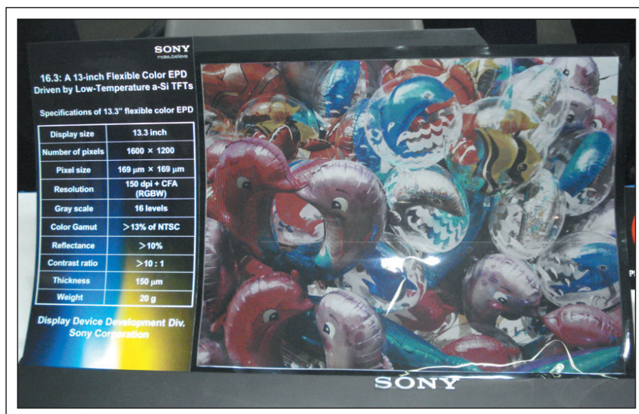
Fig. 1: Sony's 13.3-in. flexible prototype uses E Ink's new color imaging technology, Triton.
