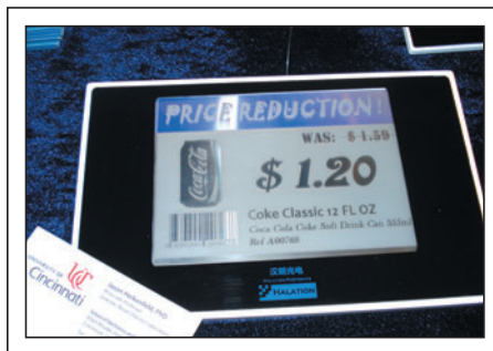
Fig. 5: Halation's smectic-A e-Paper displays exhibit good e-Paper performance with the potential for low-cost manufacturing.
