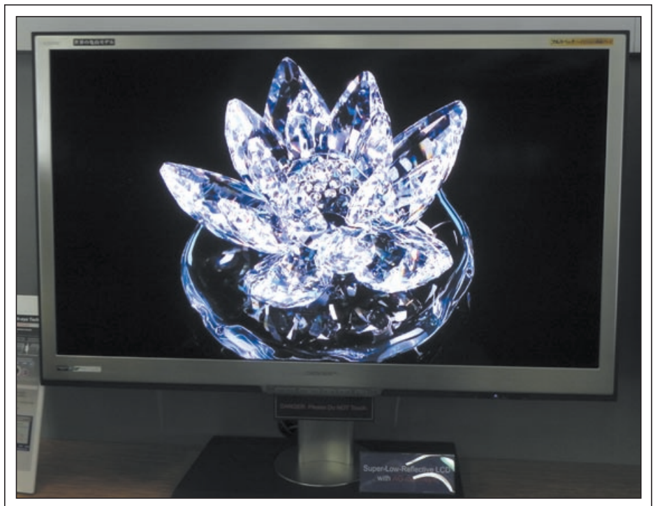
Fig. 5: Using the technology based on moth-eye structures, Sharp has developed a new anti-reflection film that yields impressive results. Photo courtesy Alfred Poor.
