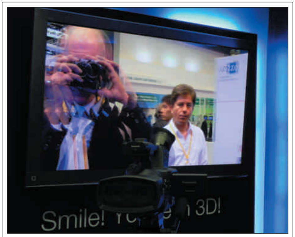
Fig. 1: The Panasonic professional 3-D camera can capture stereoscopic images in real time; see the double image of this article's author as he took this photo. Photo courtesy Alfred Poor.
