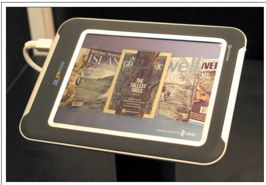
Fig. 1: Qualcomm exhibited color and monochrome 5.7-in. XGA displays built with its mirasol® MEMS technology.
