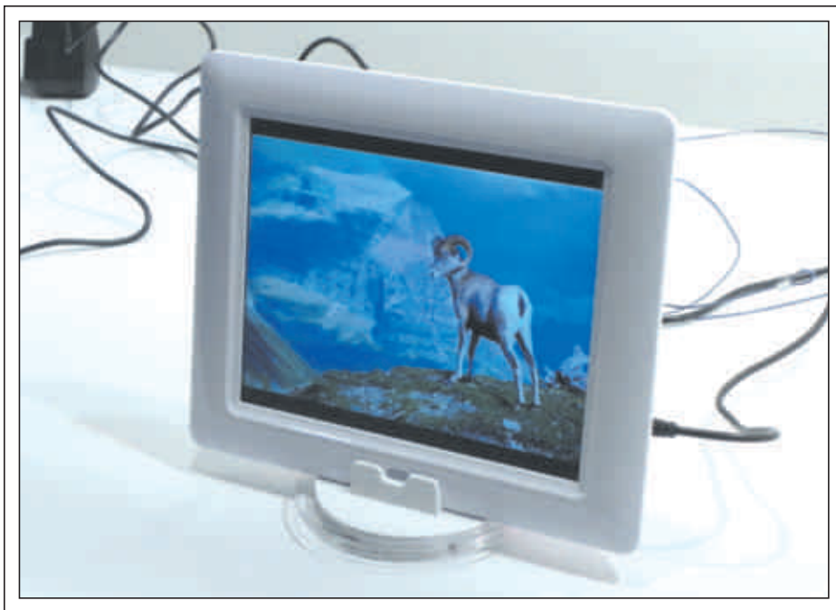
Fig. 2: The autostereoscopic photo frame by Newsight Japan creates five views of a scene so that you can "see around" objects in the foreground. Photo courtesy Alfred Poor.
