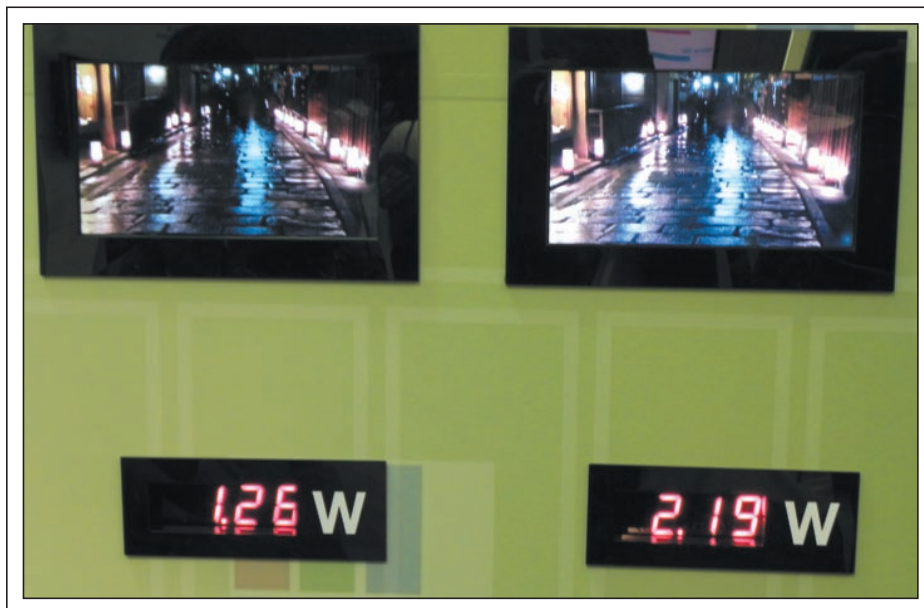
Fig. 2: The PenTile® pixel structure of Samsung's demonstration panels uses less power than that of a conventional LCD panel with equivalent resolution. Photo courtesy Alfred Poor.
