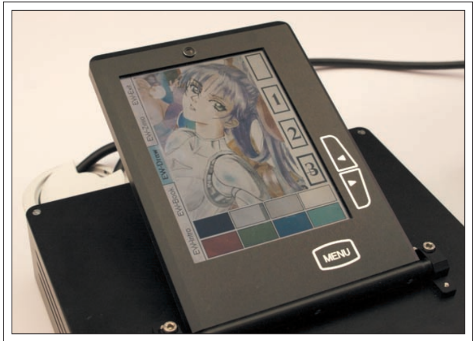
Fig. 2: Liquavista's e-reader prototype display achieves color via a color-filter array atop a monochrome electrowetting medium. Future generations may use a color-sequential backlight instead.
