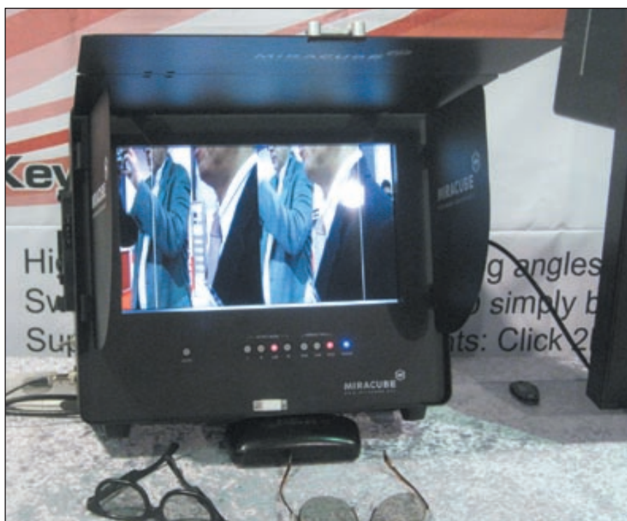
Fig. 3: This viewfinder from Miracube for a 3-D camera system is based on micropolarizer technology and passive glasses.
