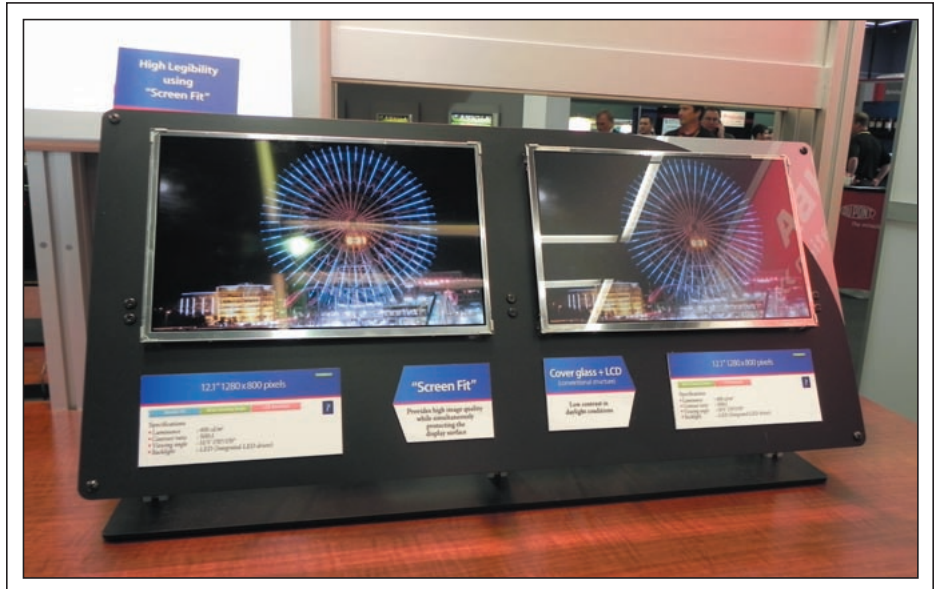
Fig. 4: The panel on the left uses Toshiba's Screen Fit technology to reduce reflections; note how the bright overhead lights are much less visible on the left-hand panel and how much the image on the right is washed out by the ambient lighting conditions. Photo courtesy Alfred Poor.
