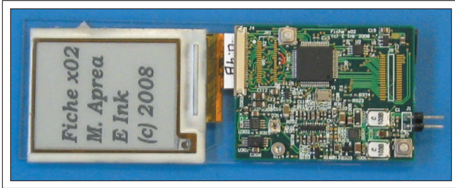
Fig. 4: In a prototype, a 1.9-in.-active-area-diagonal display appears on the left. The large IC shown on the top is an NXP LPC2148 ARM7 processor. Much of the circuitry on the bottom half of the board generates display supply and bias voltages. The board is the same size as the display, measuring roughly 2 x 1.5 in., so that the board can be folded beneath the display for compactness.
