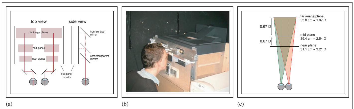
Fig. 3: Fixed-viewpoint volumetric display. (a) Schematic of viewports in the display and optical paths to the eyes; the left side is a view from the top and the right side is a view from the right. (b) A viewer using the display. The head position is fixed with a bite bar. (c) Schematic of image-plane spacing.
