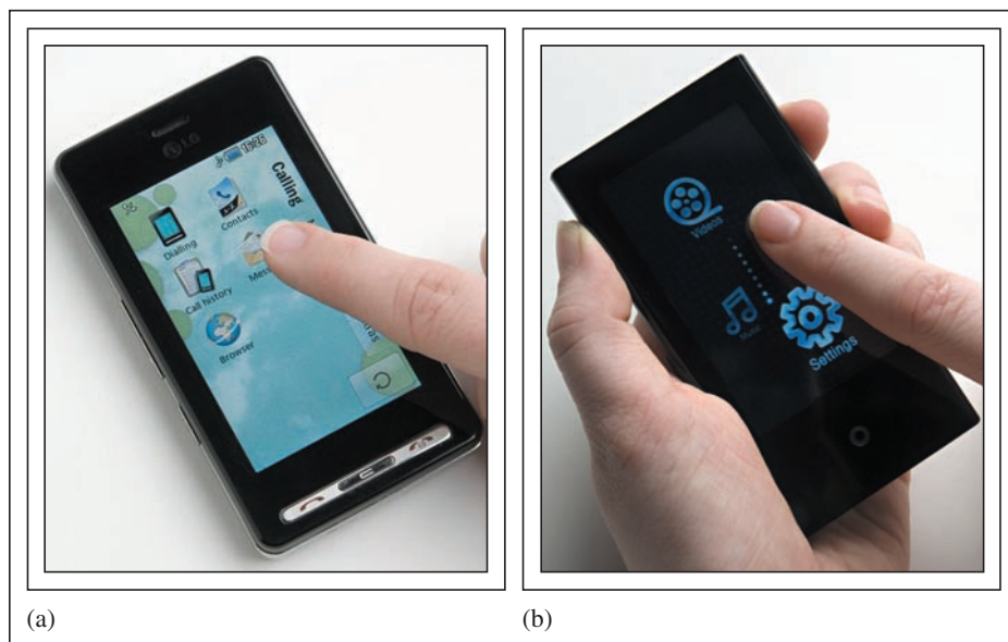
Fig. 1: The LG Prada phone (a) and the Samsung Yepp YP-P2 media player (b) are two of the first consumer-electronics products to use projected-capacitive touch screens.
