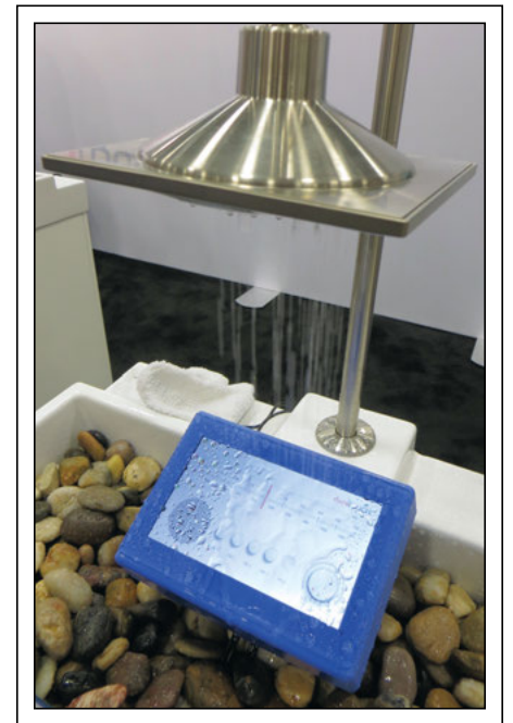
Fig. 4: UICO's fun demonstration of water-resistance for p-cap touch was about as graphic and clear as it could be. UICO achieves this very high level of water resistance by writing its own touch-controller code, but similar results have been accomplished by the major suppliers. Photo courtesy Geoff Walker.
