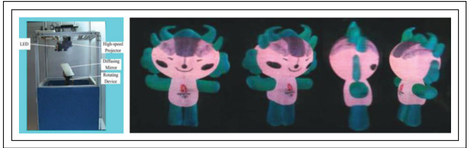
Fig. 6: Above are shown the 45°-tilted special-diffusion screen technique implemented by Zhejiang University (left) and views from different angles of a 3-D image displayed by the system (right).
