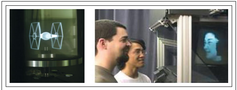
Fig. 5: Above are two different views of the 45°-tilted special-diffusion screen technique as implemented by the black-and-white 3-D light-field display from Jones's system.
